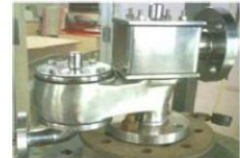
PRESSURE & VACUUM RELIEF PIPE AWAY
