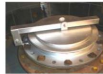
EMERGENCY RELIEF MANHOLE COVER
